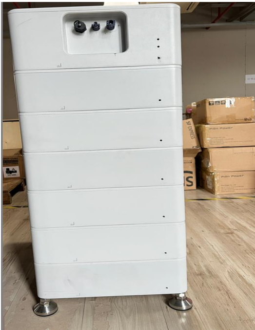
Figure 3: Side View of BESS unit
